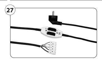
Open the terminal contacts by pressing the plungers and connect all of the wires of the motor cable
