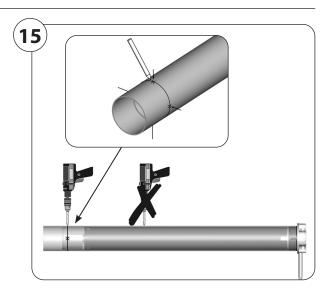
**5.** Screw or rivet the precision tube to the drive adapter **(8)**.
