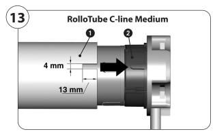
**3.** Slide the tubular motor into the precision tube.
