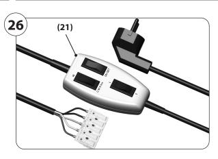
1. Open the terminal contacts by pressing the plungers and connect all of the wires of the motor cable (15) with the same colours and corresponding to their functions, see also figure [23].
