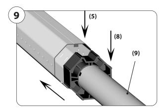
2. Subsequently, press the winding shaft (5) fully onto the adapter (10).
