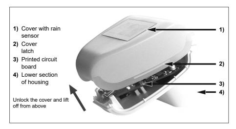
The cover of the DuoFern Environmental Sensor with the rain sensor is latched at the lower edge on the left and right (see Fig.). Remove the cover from the DuoFern Environmental Sensor. Proceed carefully to avoid tearing off the cable connection between the printed circuit board in the lower section and the rain sensor in the cover.
