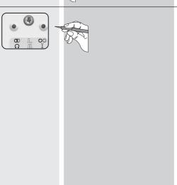
Release the "Disconnect button" as soon as the status LED lights up red continuously.
