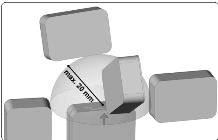
Check that the sensor part and magnet fit into the window frame. You can find the dimensions in the technical specifications on page 9. Alternatively, we recommend an installation on the window frame.
