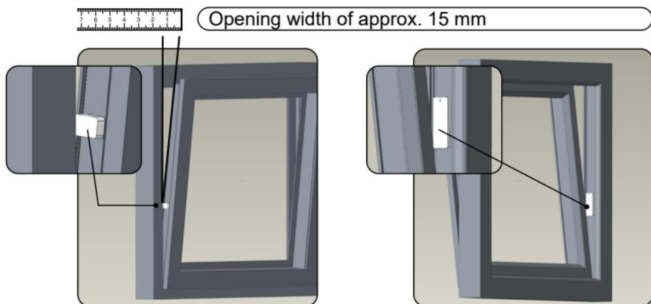
The magnet is attached to the handle side of the window sash.
