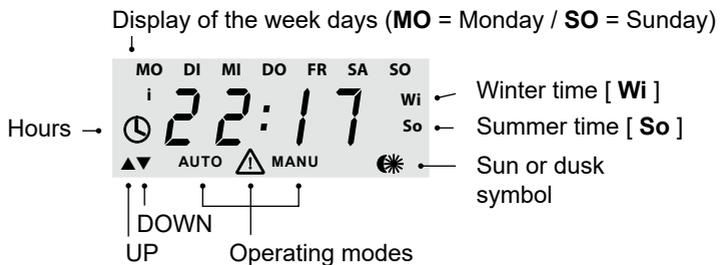
The Modi Belt Box Timer is used for connecting and controlling tubular motors and can be installed in existing belt boxes.
