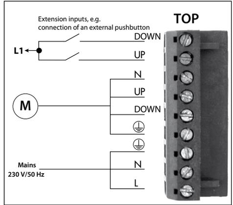
**Insert the connector into the device after the connection is completed.**
