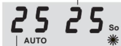
*Current measured brightness (0-29). With increasing sun, the measured value rises.*
