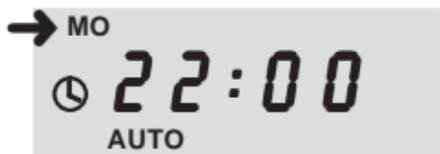
Individual every day adjustment of the opening and closing time for your roller shutter. In addition, it is possible to adjust one opening and closing time, respective, valid for all weekdays.
