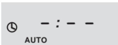
If any time appears in the display after switching on, please do carry out a software reset (see page 53) before executing further adjustments.
