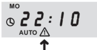
You can set the time control to random mode via the selection key for operating modes. Through this, the adjusted switching times are delayed by up to 30 minutes.
