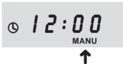
With the assistance of the selection switch for operating modes, the automatic mode can be switched off. All adjusted switching times are not effective any more. Sun and twilight functions continue to be valid.
