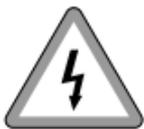
**Danger to life exists caused by electric shock.**
